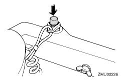
After stopping the engine, tighten the air vent screw on the fuel tank cap and set the fuel cock lever or knob to the closed position, if equipped.
